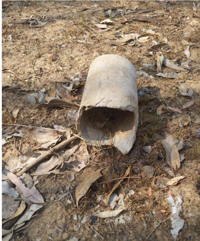
Photo 5 - Potential ACM Pipe
